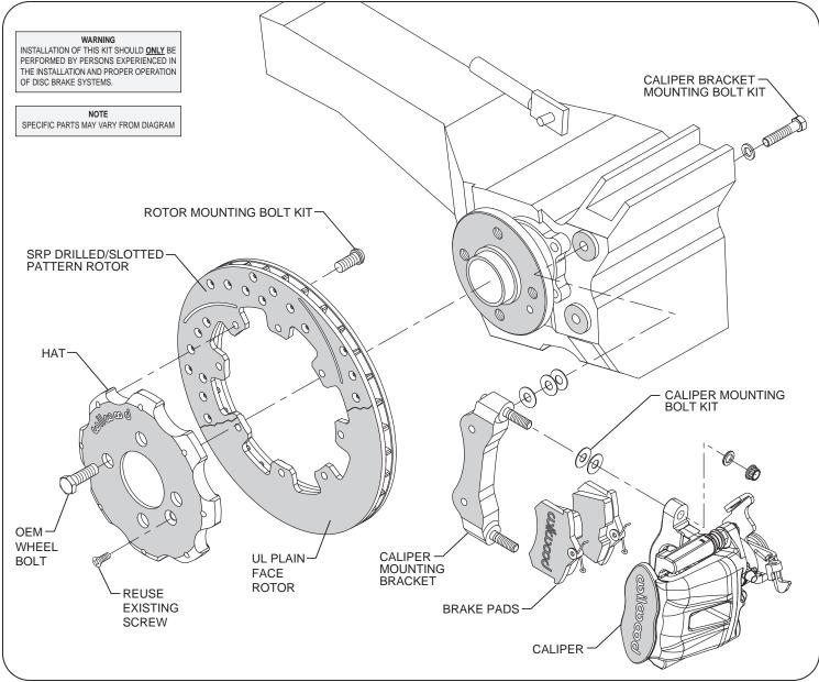
Typical Installation Diagram, Major Components Identified.
