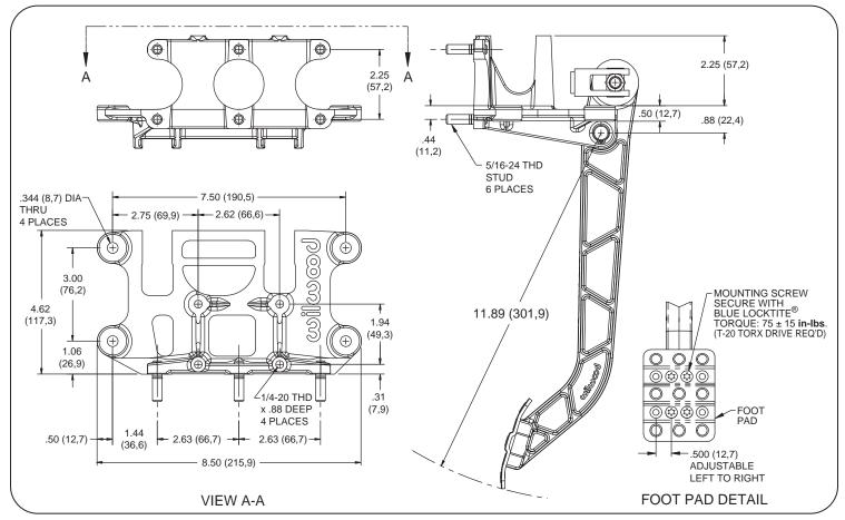
REVERSE MOUNT DUAL PEDAL ASSEMBLY, MOUNTING CHARACTERISTICS
