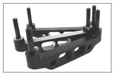
**Typical Caliper Mounting Brackets**
