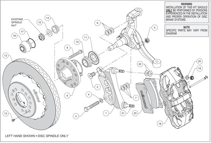
Figure 1. Typical Installation Configuration
