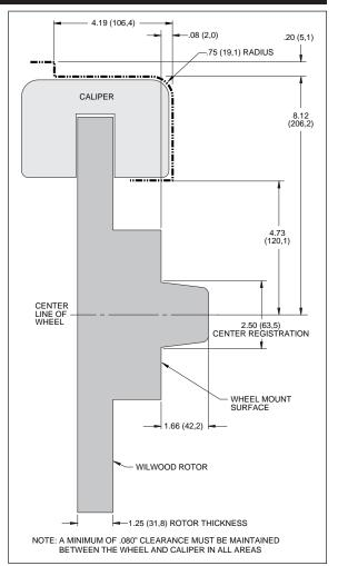
Figure 2. Wheel Clearance Diagram
