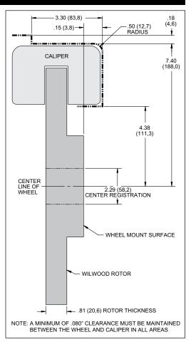
Figure 2. Wheel Clearance Diagram
