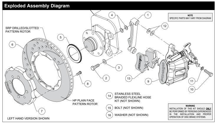
Figure 2. Typical Installation Configuration
