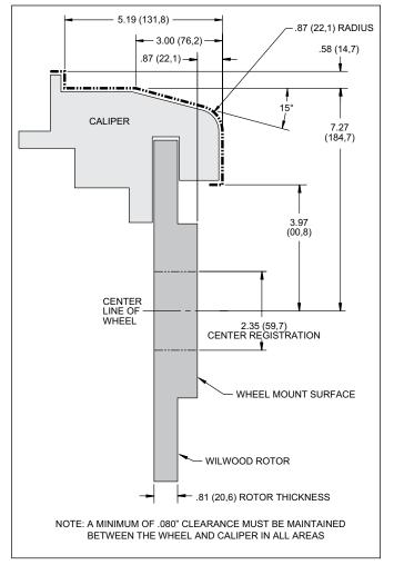
Figure 3. Wheel Clearance Diagram
