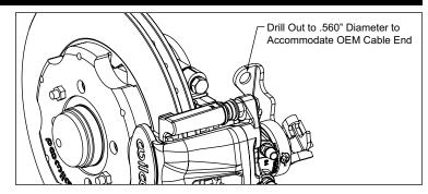
Figure 1. Caliper Cable Bracket Modification
