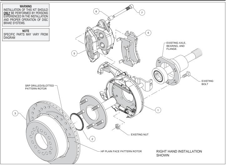
Figure 1. Typical Installation Configuration
