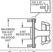
Figure 3. Axle Flange Maximum Dimension
