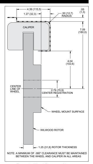
Figure 2. Wheel Clearance Diagram
