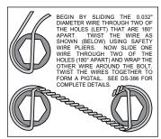
Figure 4. Safety Wire Diagram
