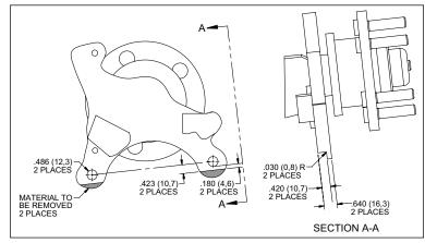
Figure 3. Spindle Modifications
