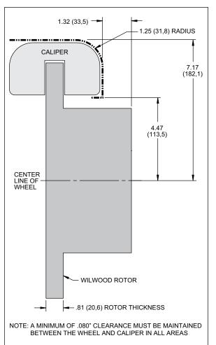
Figure 2. Wheel Clearance Diagram
