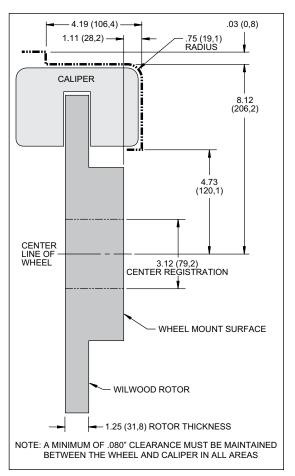
Figure 2. Wheel Clearance Diagram
