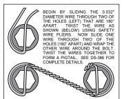
Figure 3. Safety Wire Diagram
