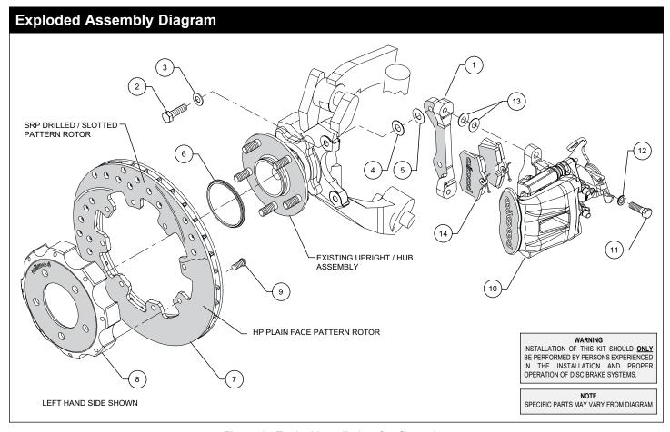
Figure 1. Typical Installation Configuration
