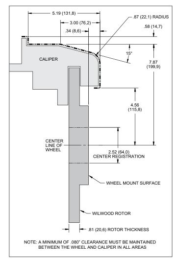
Figure 2. Wheel Clearance Diagram
