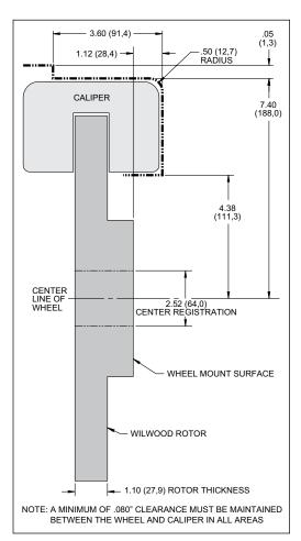
Figure 2. Wheel Clearance Diagram
