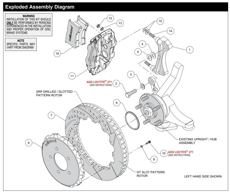
Figure 1. Typical Installation Configuration
