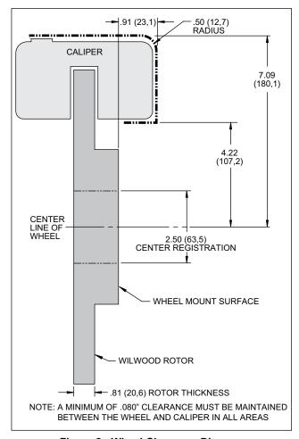
Figure 2. Wheel Clearance Diagram
