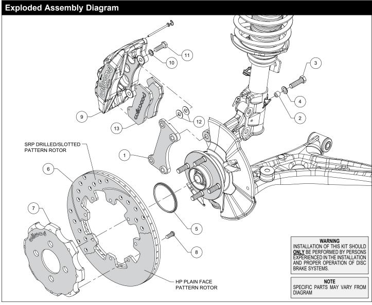
Figure 1. Typical Installation Configuration
