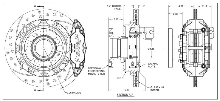
Figure 2. Kit Mounting Dimensional Characteristics
