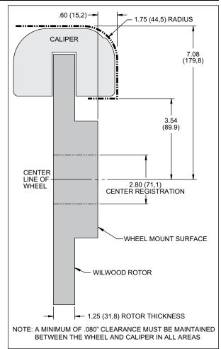
Figure 2. Wheel Clearance Diagram
