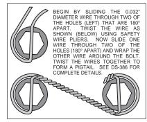
Figure 3. Safety Wire Diagram
