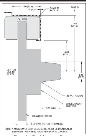
Figure 2. Wheel Clearance Diagram
