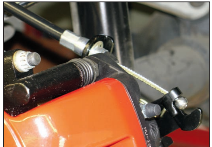
Photo 2. Installation of Cable to Wilwood Combination Parking Brake Caliper
