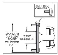
Figure 3. Axle Flange Maximum Dimension
