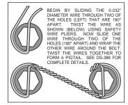
Figure 4. Safety Wire Diagram
