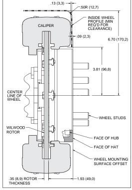
Figure 2. Wheel Clearance Diagram
