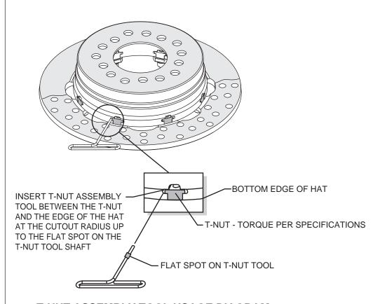
T-NUT ASSEMBLY TOOL USAGE DIAGRAM
