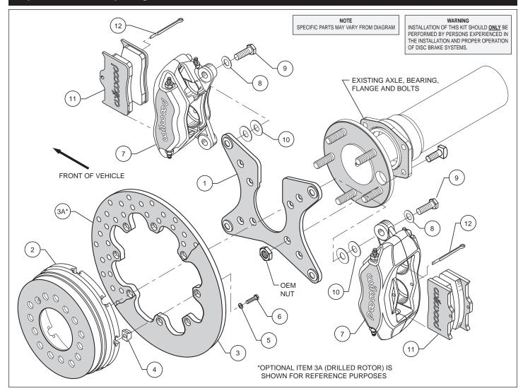
Figure 1. Typical Installation Configuration
