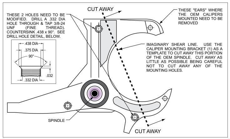
Figure 1. Steering Arm / Spindle Modifications
