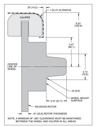
Figure 3. Wheel Clearance Diagram
