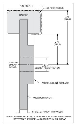
Figure 2. Wheel Clearance Diagram
