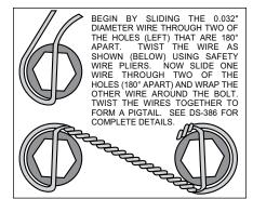
Figure 3. Safety Wire Diagram
