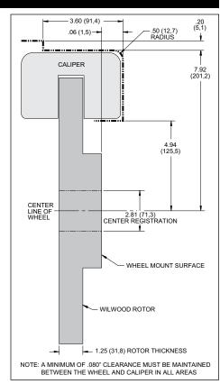
Figure 2. Wheel Clearance Diagram
