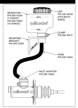
Figure 2. Remote Mounted Master Cylinder
