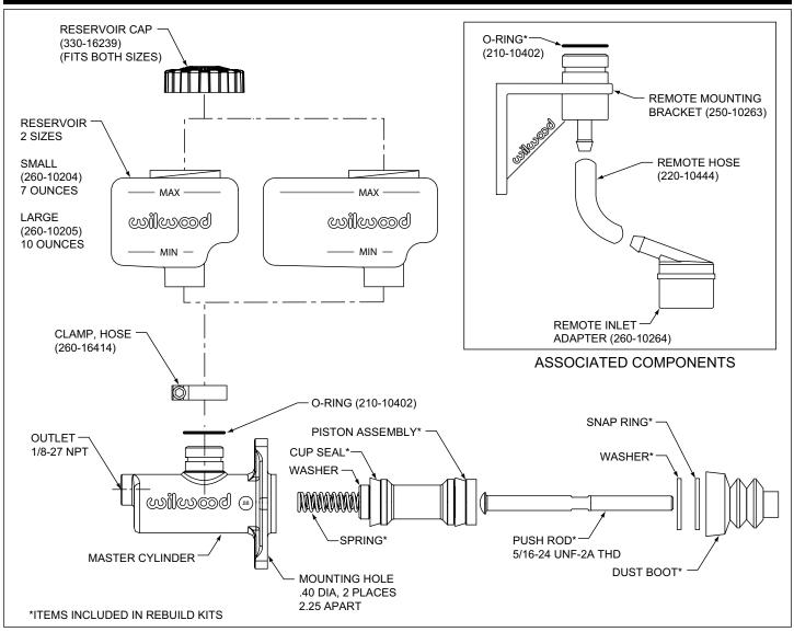
Figure 4. Master Cylinder and Associated Components
