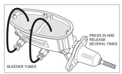
Typical Bleeder Tube Setup and Use
