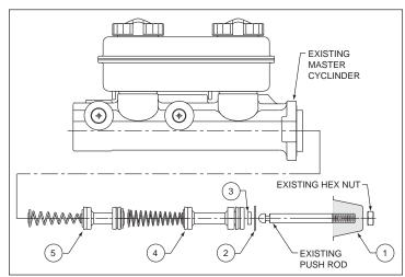
Figure 1. Tandem Master Cylinder Rebuilding Assembly Diagram
