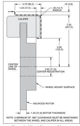
Figure 2. Wheel Clearance Diagram
