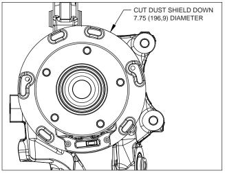
Figure 3. Backing Plate / Dust Shield Modifications
