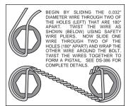
Figure 4. Safety Wire Diagram
