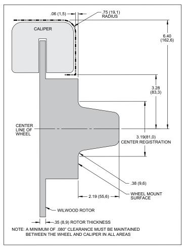
Figure 2. Wheel Clearance Diagram
