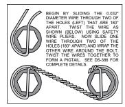
Figure 4. Safety Wire Diagram
