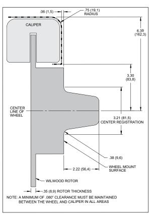
Figure 2. Wheel Clearance Diagram
