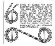
Figure 4. Safety Wire Diagram
