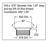
Figure 3. Drill and Tap Detail
