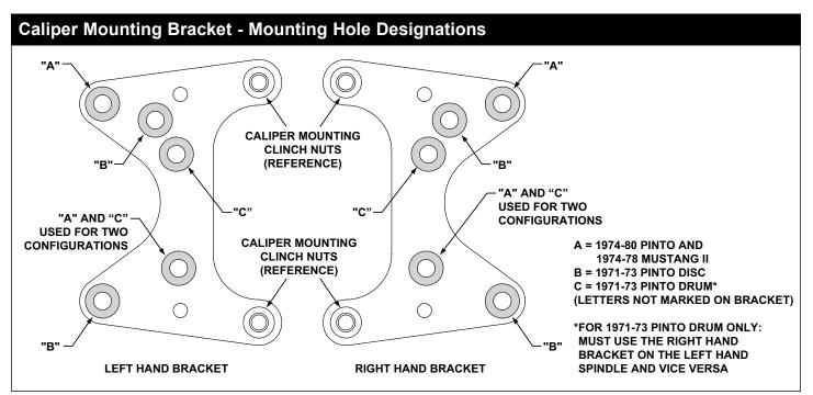
Figure 1. Wilwood Caliper Mounting Bracket
