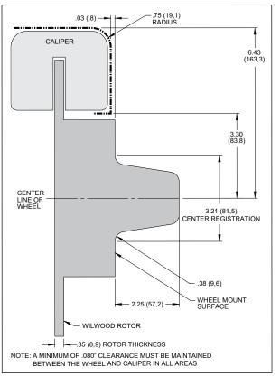
Figure 3. Wheel Clearance Diagram
