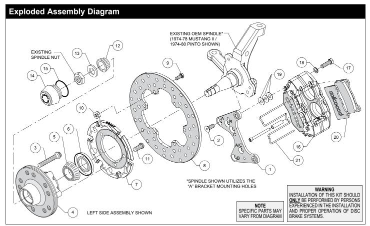
Figure 2. Typical Installation Configuration
