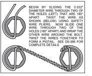
Figure 4. Safety Wire Diagram
