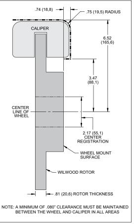
Figure 2. Wheel Clearance Diagram
