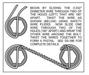
Figure 3. Safety Wire Diagram
