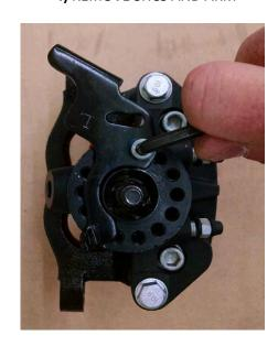
**6)** REINSTALL LEVER & TIGHTEN NUT (ALIGN SPLINES IN ARM TO SHAFT)
