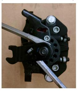
**5)** ROTATE ARM CLOCKWISE 7 (POSITIONS/HOLES) REINSTALL APPLY LOCTITE #242 TO THREADS AND TIGHTEN TO 140 IN-LBS
