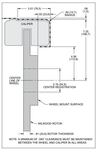
Figure 2. Wheel Clearance Diagram
