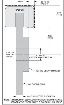
Figure 2. Wheel Clearance Diagram
