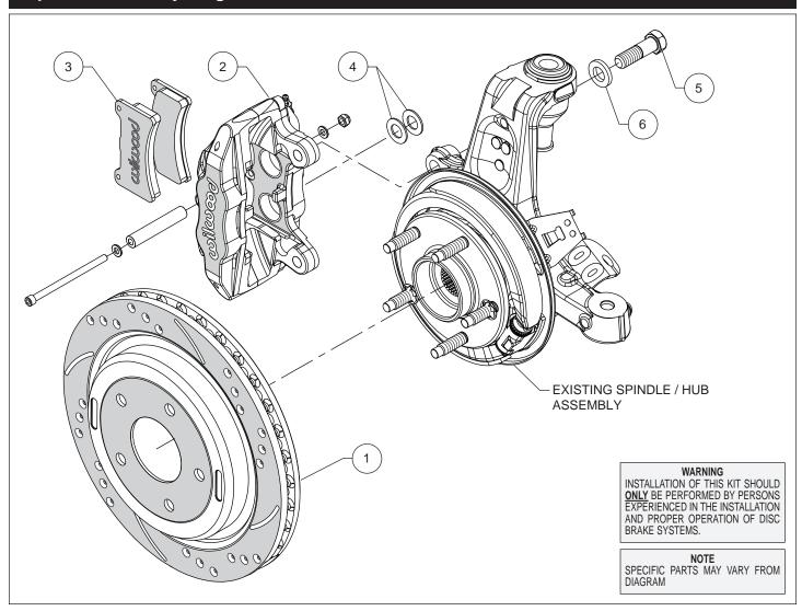
Figure 1. Typical Installation Configuration
