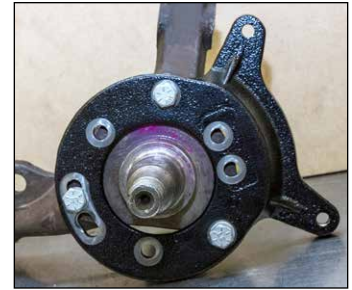
Photo 2 (3-Bolt Spindle Mounting) (R/H Side Shown)
