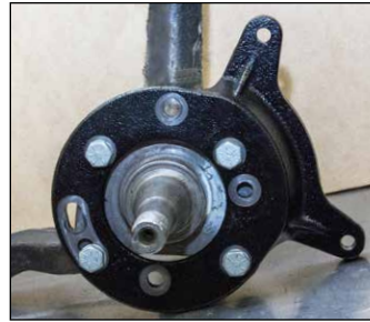
Photo 1 (4-Bolt Spindle Mounting) (R/H Side Shown)
