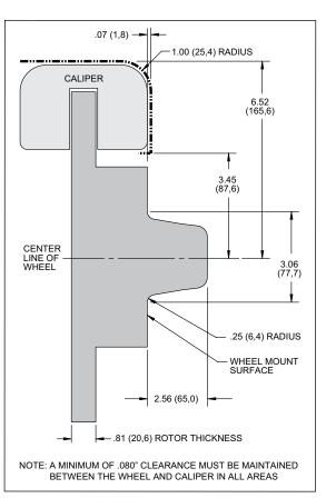
Figure 3. Wheel Clearance Diagram
