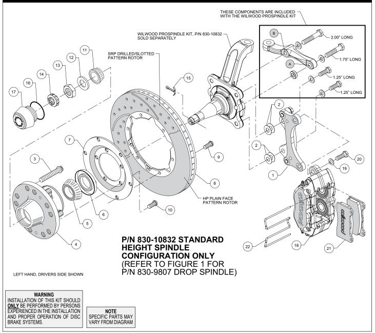
Figure 2. Installation Configuration For Standard Height Spindle, P/N 830-10832
